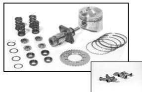
Hardfaced cam (HF) on billet core. New needle bearing cam (NB) no core needed. Machine customer cylinder head 127-HD for (NB) cam. Rocker arms (127-RA) weld and grind/cost each cust cores. #127-02 Slotted cam sprocket.
