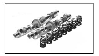
Hardfaced (HF) cams, per pair, on customer cores. #40-0893 K.P.M. valve springs to .425" lift. #40-4089 K.P.M. valve springs to .475" lift. #40-1008 K.P.M. titanium tops (use for 40-4089). #40-1013 K.P.M. cam buckets (shim under 650/750). #305-K R/D 750 KZ/GPZ valve spring kit. Wiseco 101/4:1 K-700 for 650 and K-810 kit for GPZ, KZ-750 (3mm o/s). W-2486 for 650, or W-3163 for 750 head gaskets.
