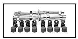
Hardfaced cams per pair, on customer cores. #40-1016 K.P.M. valve springs.
