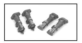
Set of 4 cams hardfaced on stock customer cores. #669-MECH remove and replace decomp. mechanism.
