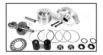
New billet/hardfaced cam with bearing on 1 end.
