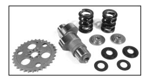
Hardfaced cam, on customer core.
